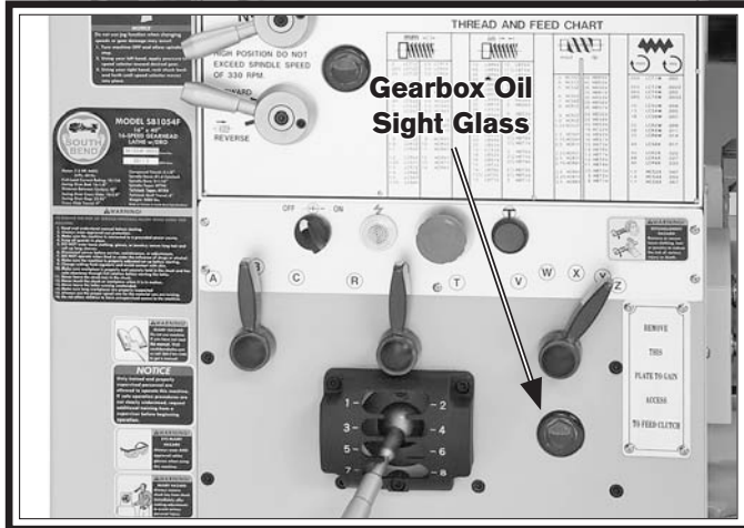
Figure 108. Location of quick-change gearbox oil sight glass.
